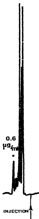
Fig. 4. Chromatogram of extract of plasma spiked with 0.625 \mu\text{g/ml} moxalactam (*) (a.u. = 0.02, injection volume = 50 \mu\text{l} ).
